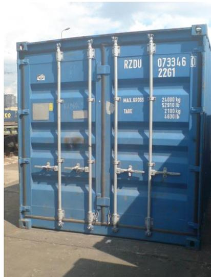
**Seal must be fixed on the main beam**
