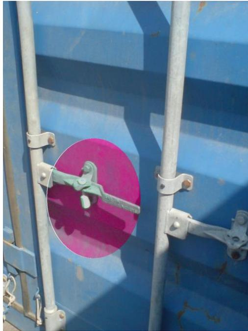
**All fasteners must be closed and fixed**
